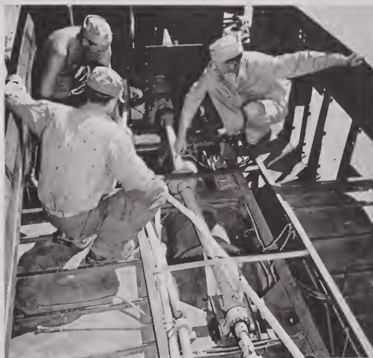
FIGURE 6. Cutaway model used at Oahu DUKW school to demonstrate many features not easily visible on ordinary production vehicle.
